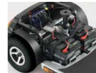
Built in anti-splash guards protect the electronics and transaxle from dirt & water damage
